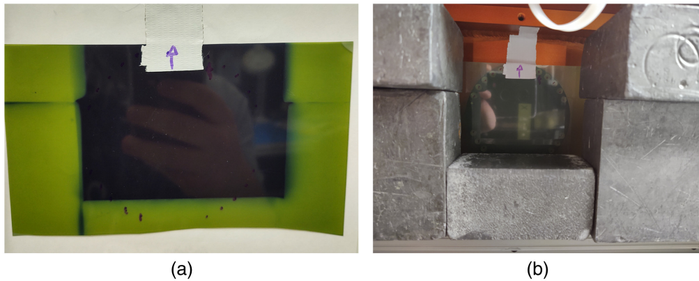
Fig. 8 Radiochromic film after it was used to verify the alignment and beam profile (a) and the film taped on the dewar port before calibration (b).
