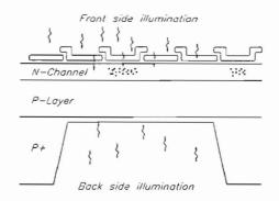
Figure 3. Cross section through a scientific imager showing three-phase polysilicon electrodes, n-channel layer (typically  $0.5\mu$ m thick and doped at  $2x10^{16}/\text{cm}^3$ ), epitaxial p-layer ( $10-12\mu$ m thick), and p+ substrate. Thinned structure illustrates back side illumination. Dots in n-channel represent collected signal electrons.
