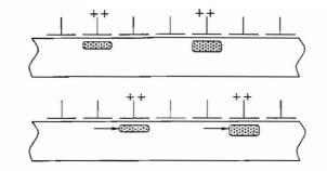
Figure 1. Simplified illustration of CCD charge transfer for a three-phase device. Changing position of positive electrode bias causes electrons in semiconductor to shift to the right.
