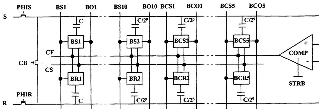
Figure 5. Binary scaled capacitor successive approximation ADC
