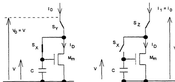
Figure 10. Current copier cell in memorize mode (left) and output mode(right).
