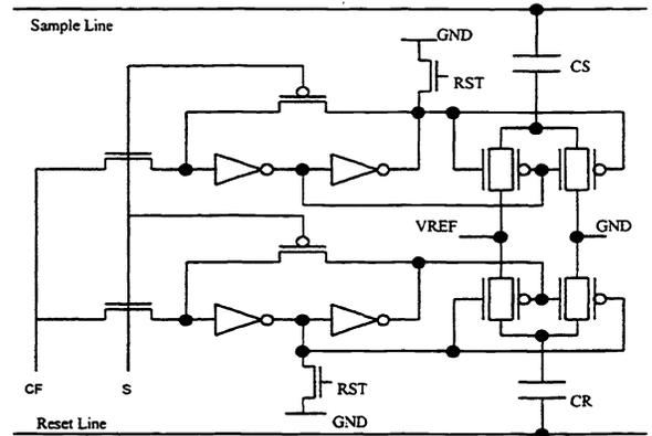
Figure 6. Bit cell latch/switch to the capacitor bottom plates for the signal and reset sides
