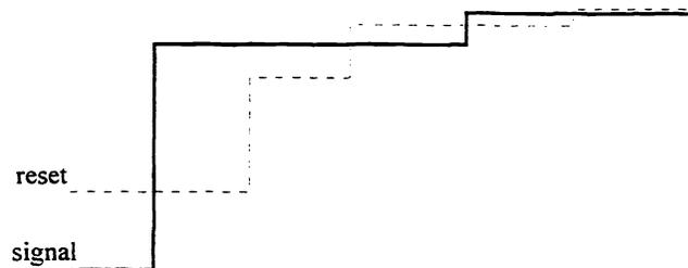
Figure 2. Internal ADC sampled reset and signal levels during conversion
