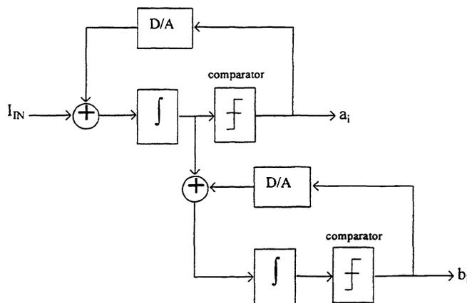
Figure 9. Block diagram of the second order sigma-delta ADC
