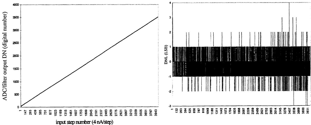
Figure 13. Transfer curve and DNL error at 5 KHz conversion rate for 12 bit incremental sigma delta ADC.
