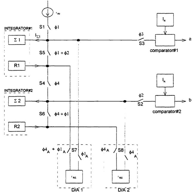
Figure 12. Current mode sigma-delta ADC
