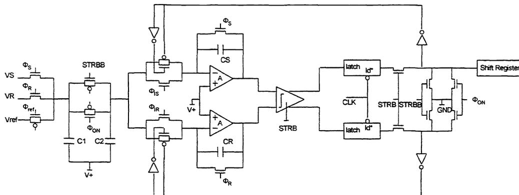
Figure 3. Successive approximation ADC circuit using switched capacitor integrators
