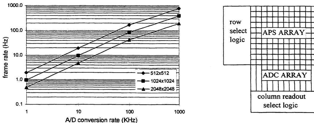
Figure 1. Frame rate vs. ADC speed for a 512x512, 1024x1024, and 2048x2048 APS with the above column parallel architecture for focal plane A/D conversion (1.5  $\mu\text{sec}$  row access time assumed).
