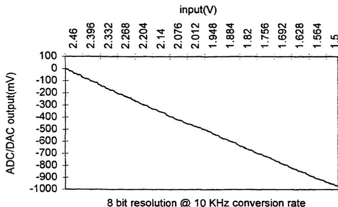
Figure 4. Transfer curve for a successive approximation ADC implemented with switched capacitor circuits.
