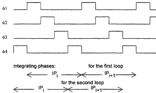
Figure 11. Sigma delta timing
