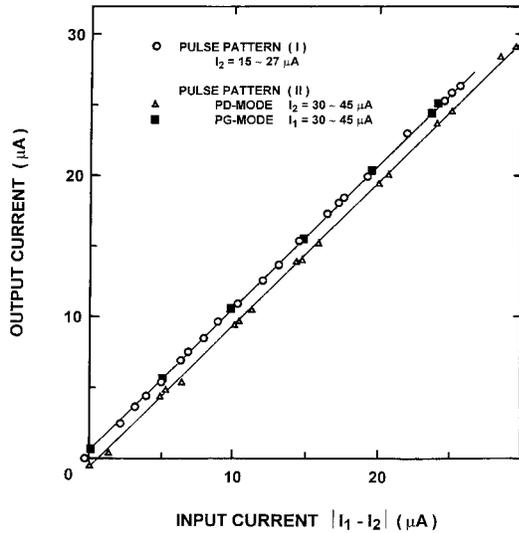
Fig. 4. Transfer characteristics of the FPN suppression circuit.
