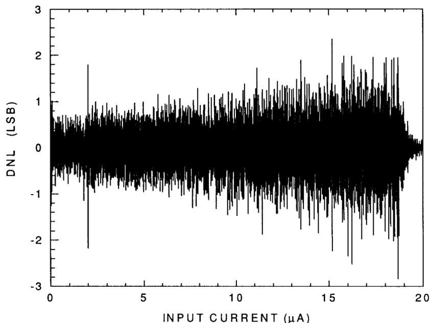
Fig. 11. Differential nonlinearity error for the 12-resolution operation.
