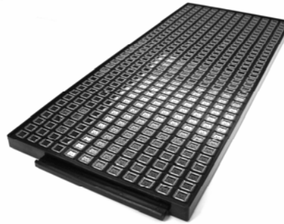
Figure 5. Photograph of 432 packaged MEMS Stages on a tray.
