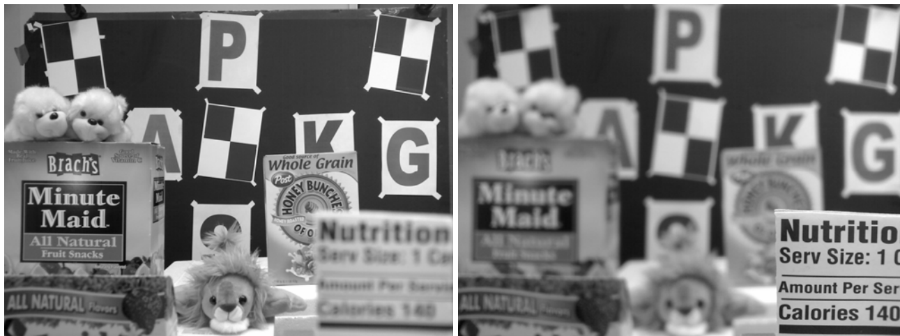
Figure 8. Photographs taken with a 2 MP MEMS digital camera of a scene with objects at various distances from the camera, focused on the furthest objects (left) and the nearest (right).
