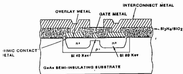
Fig. 1) The Self-Aligned Gate FET (after N. Doudoumopoulos, Hughes Aircraft Company, used with permission).
