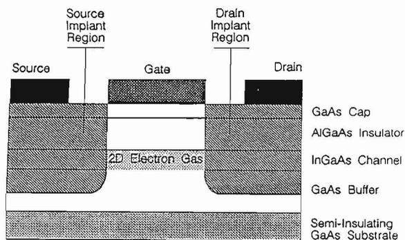
Fig. 2) The Complementary Heterojunction Field Effect Transistor (CHFET).
