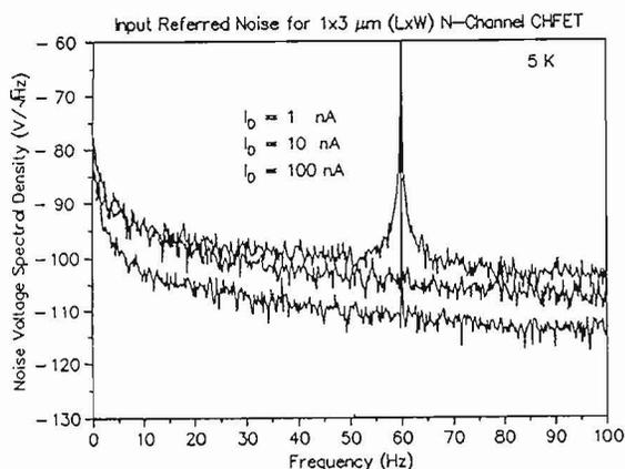
Fig. 5) The input referred noise in a 1x3  $\mu\text{m}$  (Lxw) CHFET at subthreshold drain currents.
