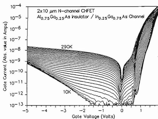
Fig. 4) The gate current in a CHFET with temperature as a parameter.
