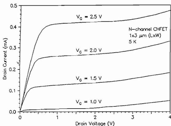
Fig. 3) The transistor curves of the CHFET.
