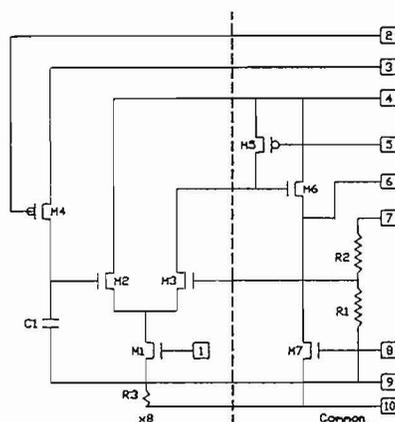
Fig. 6) The Switched Follower 8x1 multiplexer based on GaAs CHFET technology.
