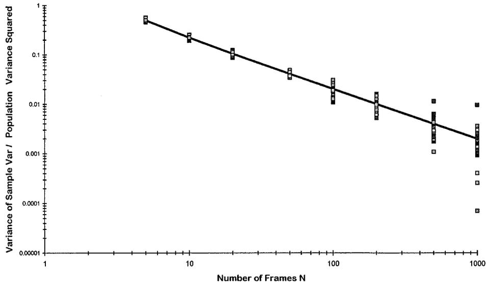
Fig. 3. Variance of the sample variance as a function of  $N$ . The line is the theoretical dependence given by Eq. (16). The data are derived from 5000 samples for each of 25 detector elements.
