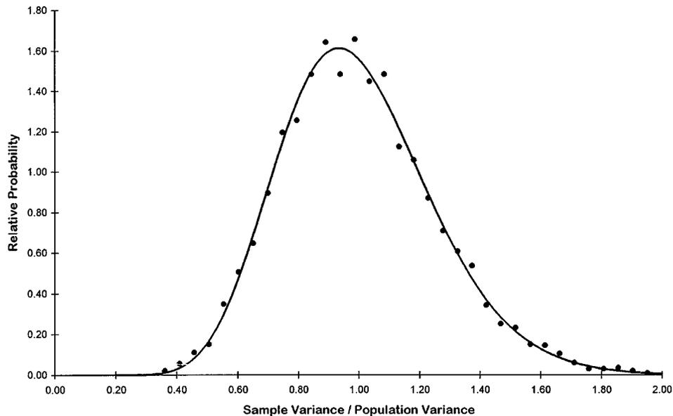
Fig. 2. Histogram for 32 frames of a  $64 \times 64$  detector array. Superimposed on the 34-bin histogram is the probability density function for the normalized sample variance [Eq. (11)].
