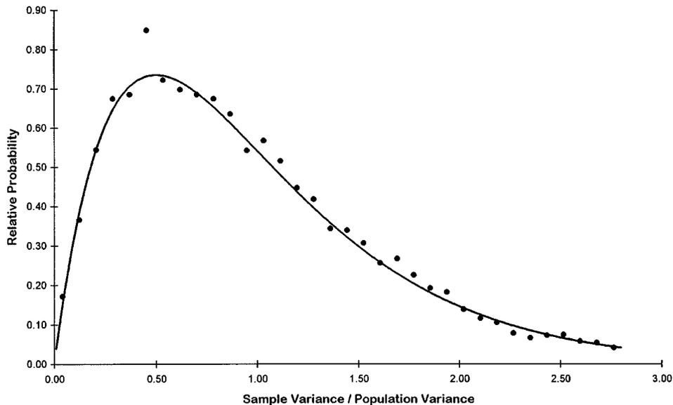
Fig. 4. A 34-bin histogram for five frames and the corresponding probability density function for the normalized sample variance [Eq. (11)]. The data are derived from 1000 five-sample sets for each of six detector elements.
