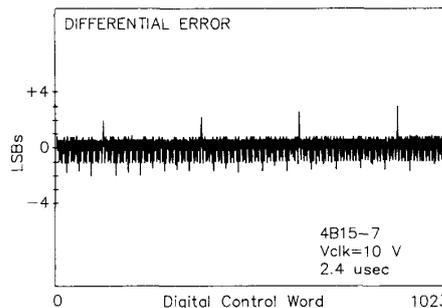
Fig. 4. Differential linearity error of pipeline circuit. Note that the 1-LSB tic mark corresponds to 1/1024th of full scale.
