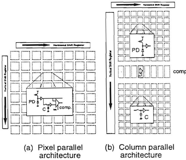
**Figure 6. Description of the architecture for on-sensor-compression**
