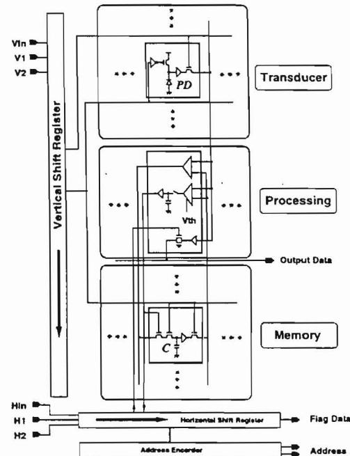
**Figure 15.** Block diagram of column-parallel-type sensor
