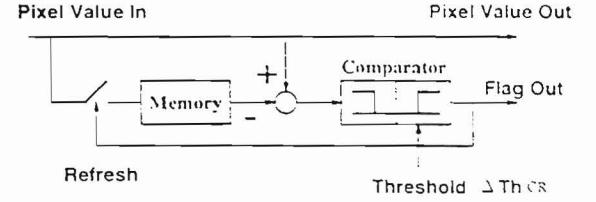
Figure 1. Description of coding algorithm in each pixel by conditional replenishment
