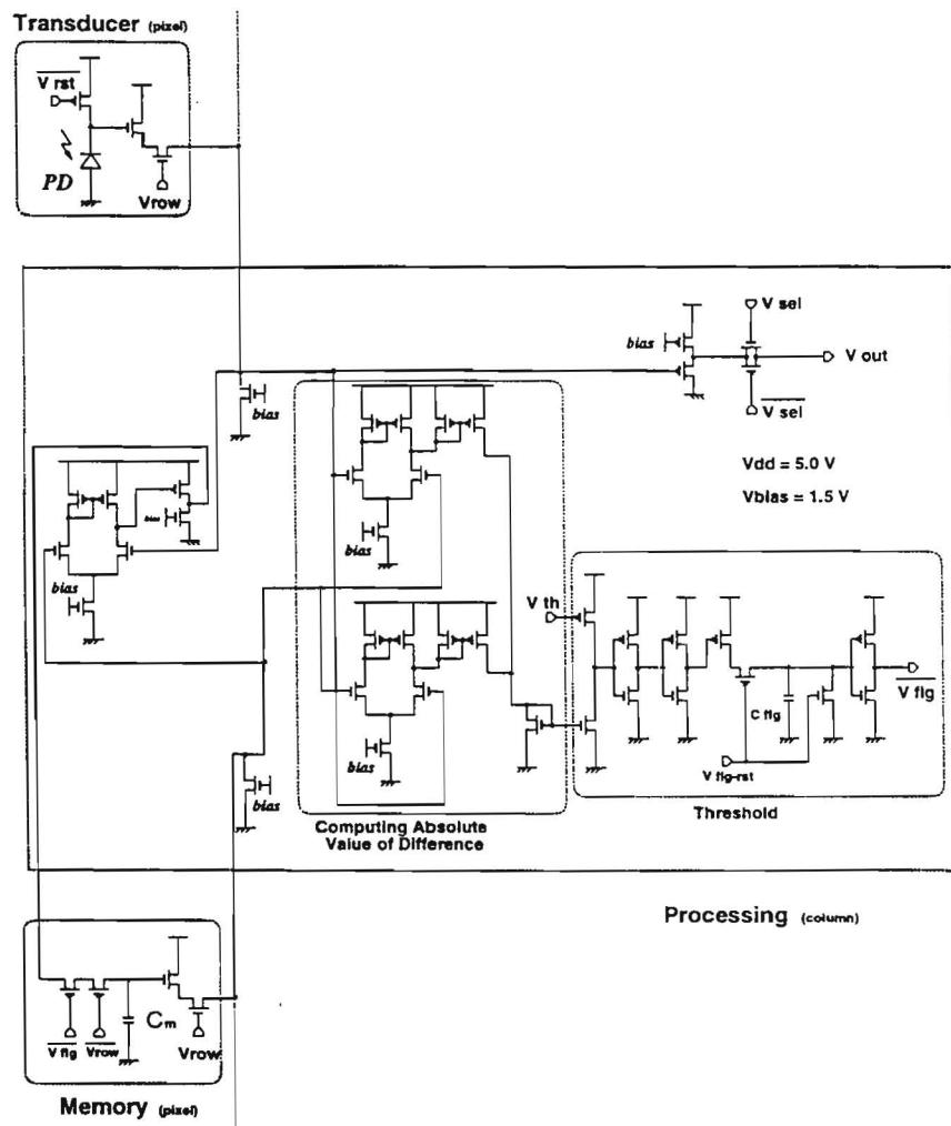
**Figure 14. An analog circuit of a pixel for column-parallel-architecture**
