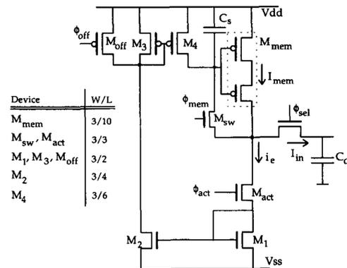
Fig. 1. Circuit diagram of the error feedback compensated current memory cell.
