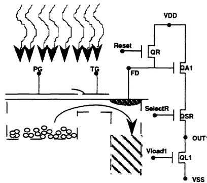
Fig. 2 Double-Polysilicon Active Pixel.
