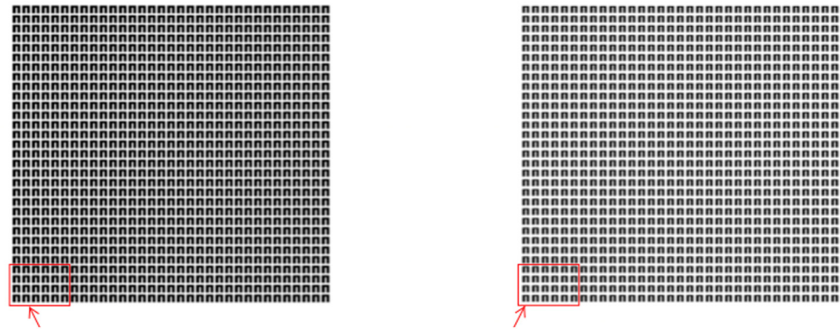
Figure A2. Zoomed-in image of each square from Figure A1 that consists of arrays of pixels in the pixel active region. Each array has different dimensions of pixel coverage.
