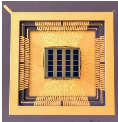
Figure 23.11 QIS test chip containing 20 different 1 Mpixel arrays designed by Dartmouth and fabricated by TSMC in a 65 nm stacked BSI CIS process. Source: Eric R. Fossum.
