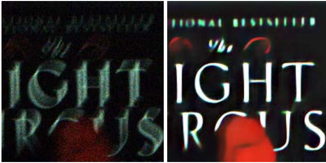
Fig. 17. Image deblurring using algorithm unrolling [156]. (Left) Input data, 14-bit 1-frame. (Right) Reconstructed.
