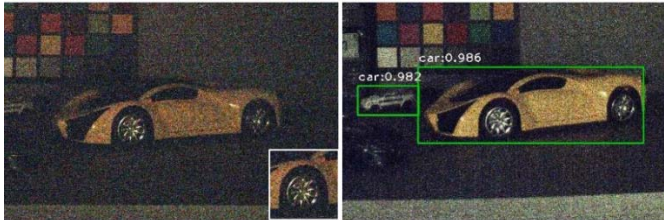
Fig. 18. Application of QIS for object recognition and tracking at a photon level of 0.71 photons per pixel. (Left) Image captured by a CIS. The detection algorithm is the current state-of-the-art Faster R-convolutional neural network (CNN). (Right) Image captured by Gigajot 16MP QIS GJ01611. The detection algorithm is based on [157]. Note the improved detection capability of the sensor–algorithm combination.
