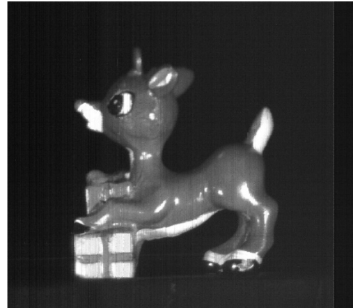
Fig. 16. Sample image acquired with 6-bit SS ADCs. Dark stripe on right side is due to covered pixels for dark reference.
