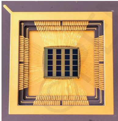
Figure 11. QIS test chip containing 20 different 1Mpixel arrays designed by Dartmouth and fabricated by TSMC in a 65nm stacked BSI CIS process.
