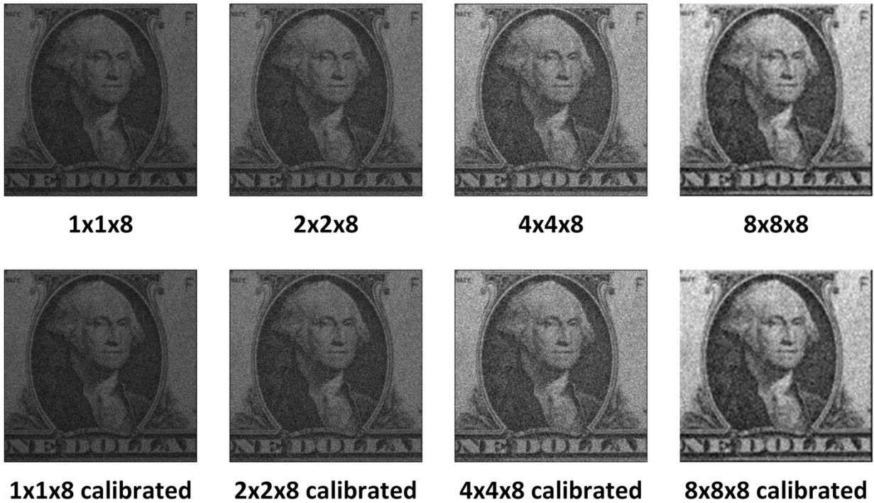
Figure 7: Comparison of images taken using the QIS camera module using either global CG calibration (normal) or per pixel CG calibration (calibrated) for different image pixel sizes.
