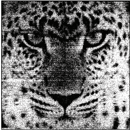
FIGURE 4. In the first image from a 1 Mjot digital single-bit QIS array operating at 1040 fps, artifacts appear from framegrabber synchronization.
