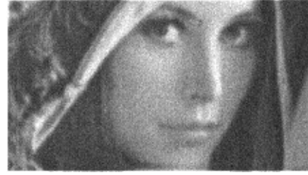
Fig. 14. Image taken with designed sensor in low-light condition (~200e-)
