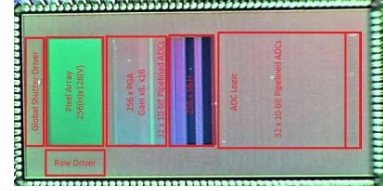
Fig. 15. Photo of the fabricated image sensor chip die
