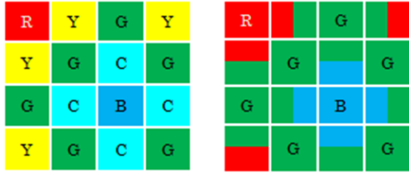
Fig.2. Transformation of the RGBCY kernel to sRGBCY showing yellow pixels composed of half red and half green filters and cyan pixels half-covered by blue and green filters.
