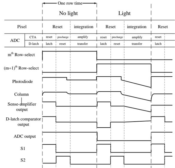
Fig. 6. Timing diagram and various phases of operation for each column and ADC.
