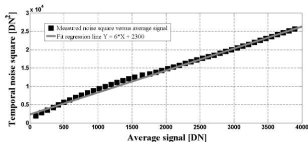
Fig 9. Measured temporal noise squared versus average signal.
