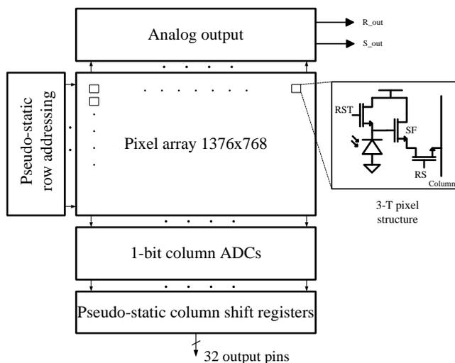
Fig. 2. Architecture of the 1MP pathfinder image sensor.
