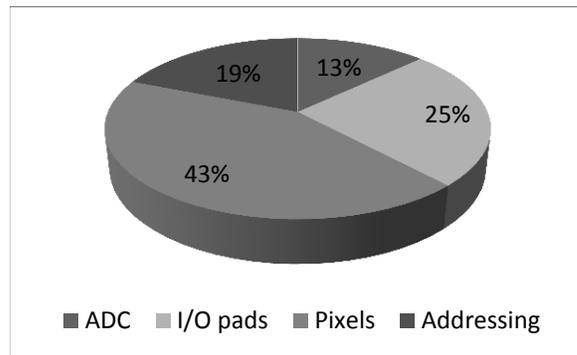
Fig. 10. Power breakdown of the imager chip.
