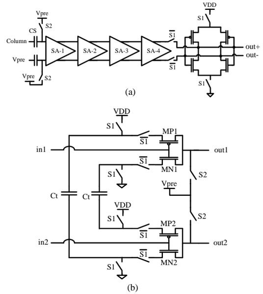
Fig. 5. (a) 1-bit ADC (shown in Fig. 4) based on a cascade of sense amplifiers and a single D-latch comparator. (b) Schematic of each sense amplifier that is implemented as a differential charge transfer amplifier.
