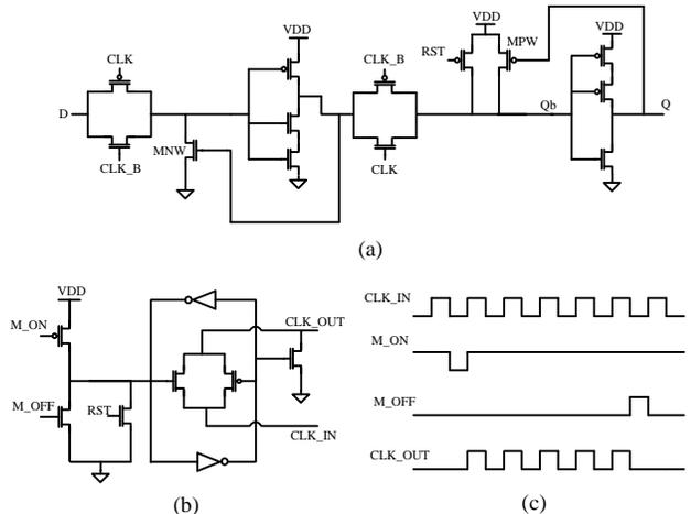
Fig 7. (a) Pseudo static flip flops and (b) clock gating units used in the row addressing and column shift register circuits, with (c) timing diagram.
