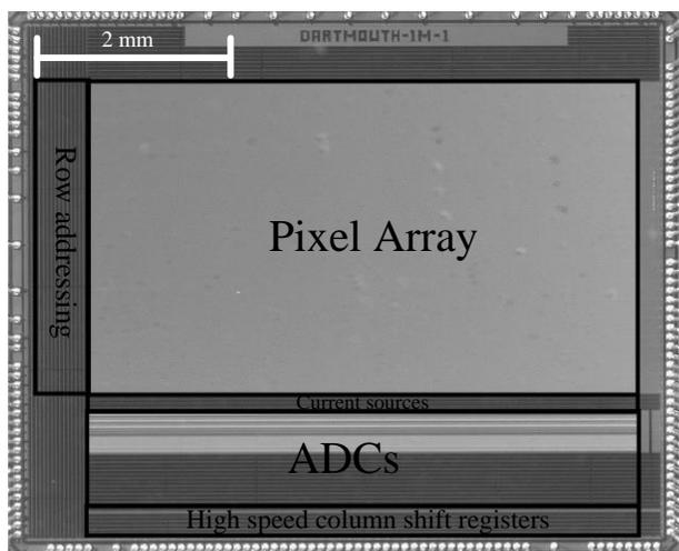
Fig. 12. Micrograph of pathfinder sensor in 0.18  $\mu\text{m}$  CMOS.
