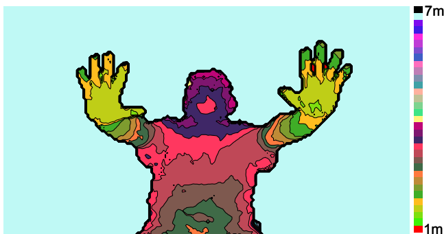
Fig. 11. A three dimensional image obtained from a human being. Not only is the distance information clearly visible, but also the image resolution is enough to resolve each finger at 1 m distance, which is important for gesture control.
