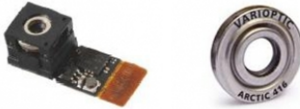
Figure 6. Photograph of a camera (left) using liquid lens from Varioptic (right).
