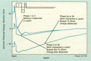
The Implantation of an Additional p Layer in phase 2, combined with appropriate biasing, would enable the application of electric fields that would steer electrons to storage sites in phase 2a or 2b.
