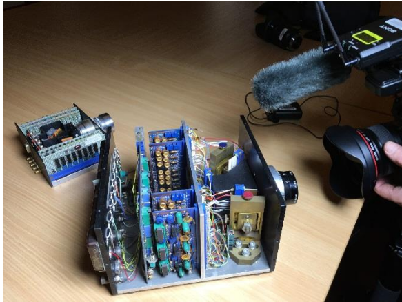
Early 70's Bell Labs CCD camera by Mike Tompsett et al.
